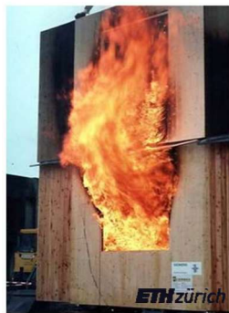
Combustible surface in fire room
