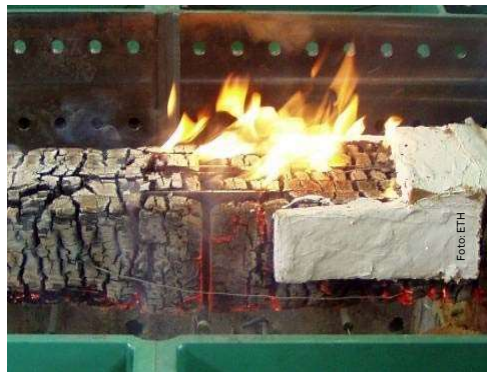
Multiple shear steel-to-timber dowelled connection
