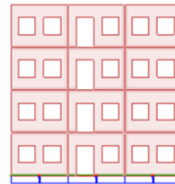
b.3 position of openings modification
