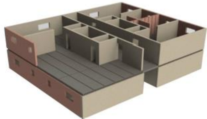
Illustration of load bearing wall structure (fib 74)
